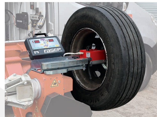
■ Wheel balancer B150.T mounted on the RGU2671.G
