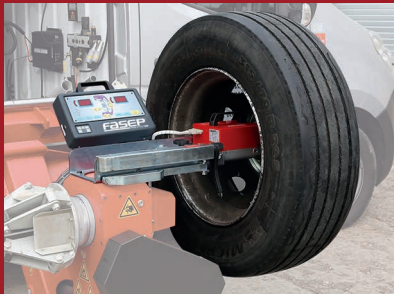
Wheel balancer mounted on RGU2671.G
