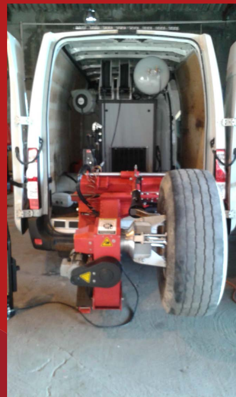
INSTALLATION AT REAR DOOR WITH INVERTED CHUCK
